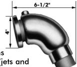
For engine installations close to the transom, (jets and stern drives) these elbows will accommodate 2" or 2½" pipe size. (Fits rectangular type exhaust manifolds only).
