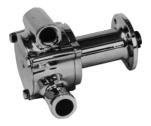
The "Magnaflow®" is a self-priming, cam driven water pump featuring chrome brass construction, friction minimizing ball bearings, long lasting ceramic seals and a tough neoprene impeller. To accommodate a variety of engine types, the "Magnaflow®" comes standard with a large 11/4" hose inlet, tapped 3/4" NPT and a pair of 1/2" NPT outlets.
