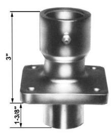
This competition rudder stuffing box uses a double seal on top and an "O" ring on the bottom, giving greater rudder shaft stability and assuring a positive leak-proof unit.
